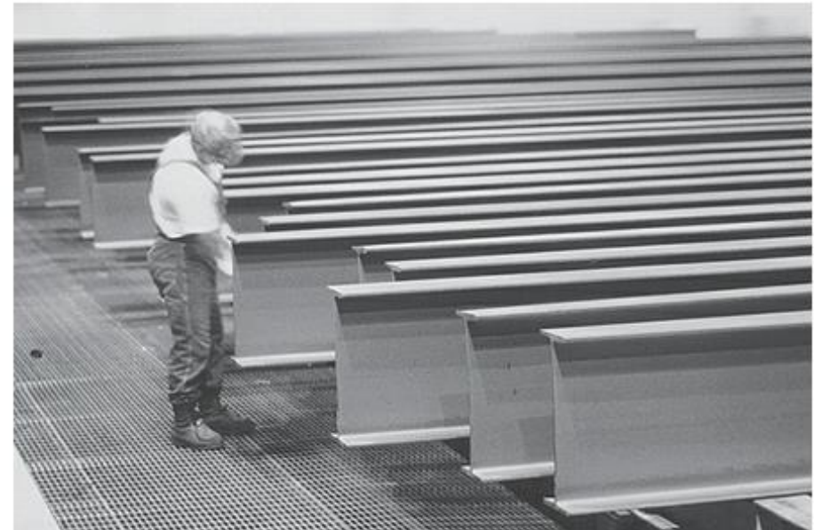
FIGURE 11.9 Wide-flange shapes are inspected for quality on the cooling bed.
