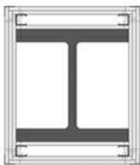
FIRE-RESISTANT BOARD ENCLOSURE
