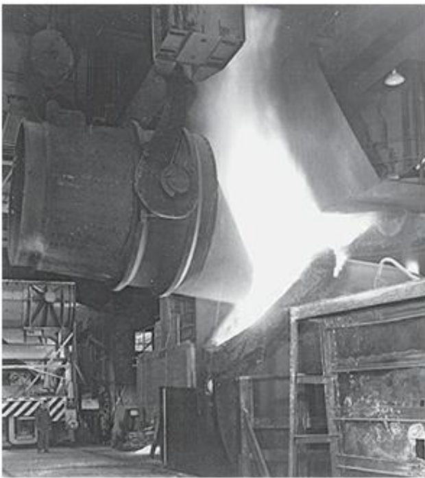
FIGURE 11.6 Molten iron is poured into a crucible to begin its conversion to steel in the basic oxygen process.
