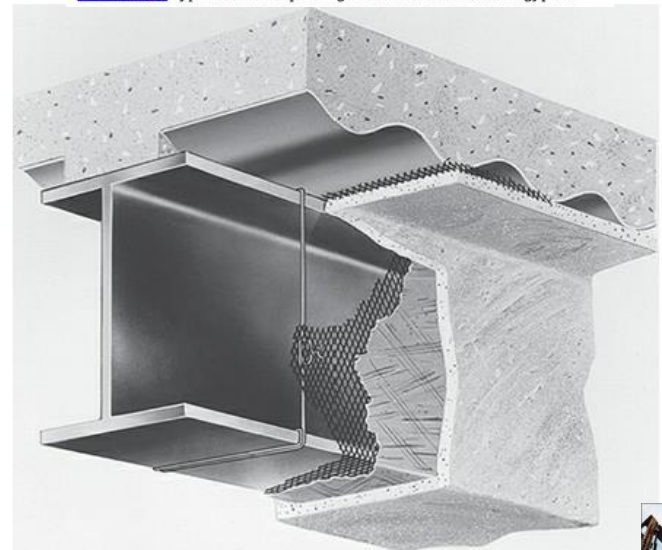
FIGURE 11.70 Lath-and-plaster fireproofing around a steel beam.
